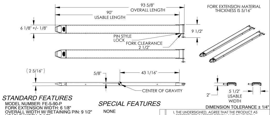
**USABLE WIDTH: 5 1/2" OVERALL LENGTH:93 5/8"** DESIGNED TO FIT 5" WIDE x 2" THICKNESS FORK SOLID STEEL CONSTRUCTION
